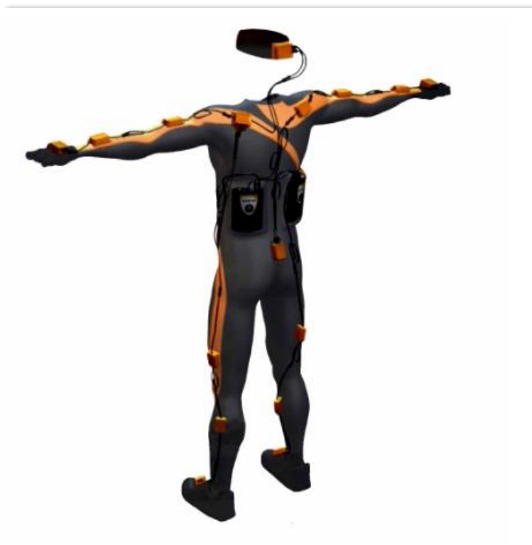
Figure I—2 Inertial Measurement Unit ( IMU ) Motion Capture System Sensor Layouts [12]
