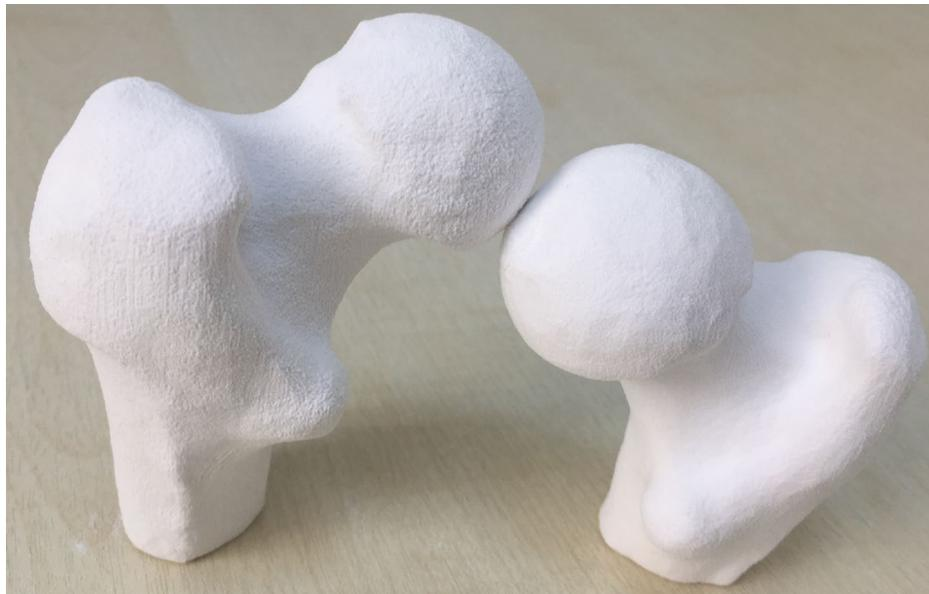
Figure 3.2: Femoral head models printed with BJ technology
