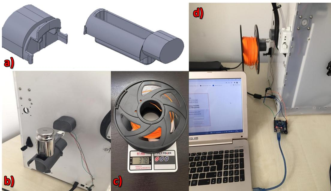
Figure 3.11: (a) 3D drawing of the filament holder mechanism, (b) Calibration of load cell with standard weight, (c) Measurement of filament weight with precision scale and validation process with the system, (d) Adaptation and operation of all parts of the system to the 3D printer
