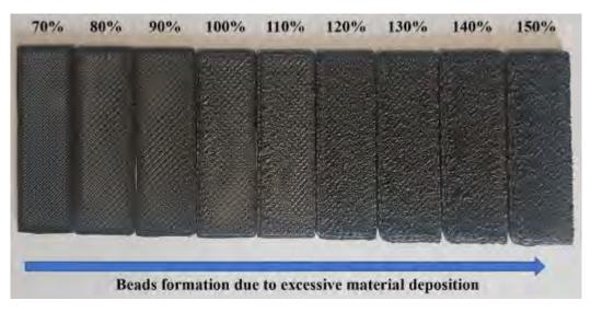
Figure 4 : Printed GPLA specimens
