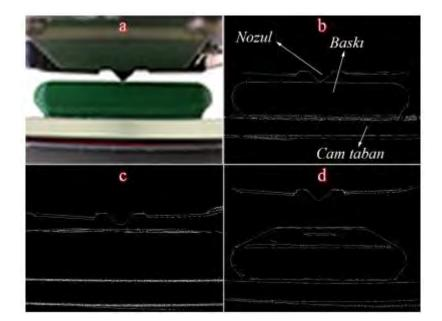
Figure 31 : The image obtained from the camera and the processed images, a) The image of the camera positioned between the nozzle and the print sample at 640x480 resolution, b) The distance between the nozzle and the print sample is quite small ( $d \le 0.06$ mm), c) The The distance approaches the threshold value ( $d \le 0.06$ mm) 0.25mm), d) The distance exceeds the threshold value (d > 0.25).
