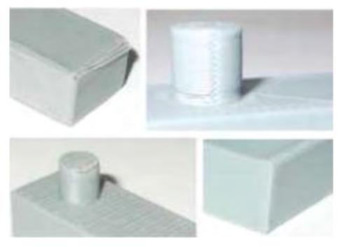
Figure 5 : Quality issues of FFF printed specimen.
