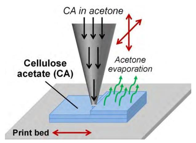
Figure 7: 3D Printing with Cellulose
