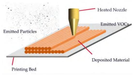
Figure 8 : Airborne emissions in FFF 3D printing.
