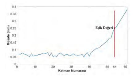
Figure 32 : Measurement of the distance between the nozzle and the print sample according to the layer number.
