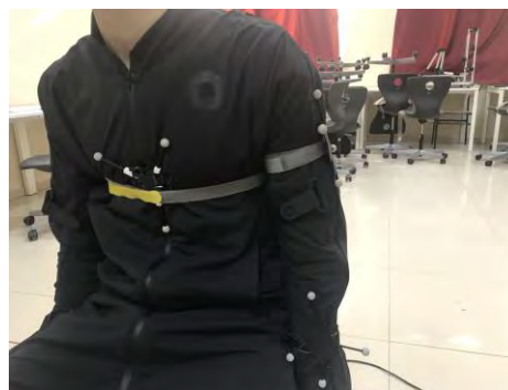
Figure 2.11: Marker positions for both Motion Capture Systems (MCSs) to import data from in vivo study.
